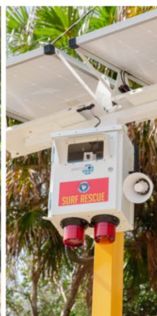
The operator will use the camera to view the emergency and monitor the situation to provide information to emergency services.
