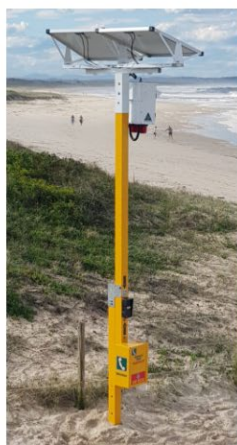
The Emergency Response Beacon (ERB) unit on the beach
